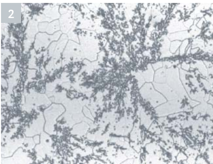
Figure 1.2: Original and impression of a mould. Ferritic cast iron with rosette-shaped arrangement of the graphite. Etched with nitric acid (3%)
